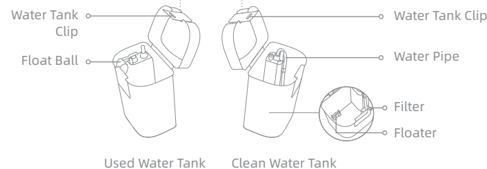
Used Water Tank
